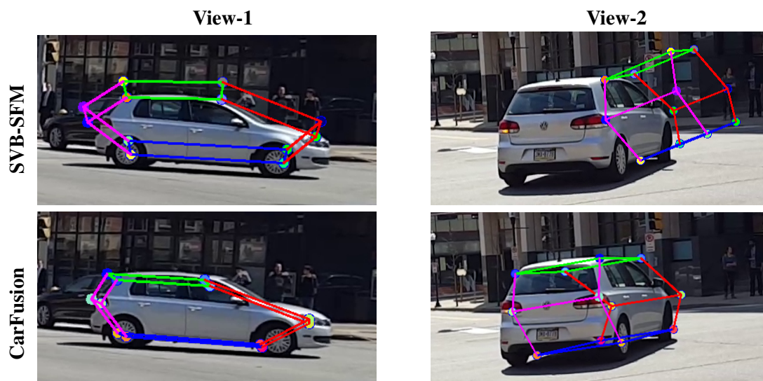
FIGURE 4.1: [Top-Left] Single-video based SFM(SVB-SFM) reconstruction of structured points. [Top-Right] The reprojection of the reconstruction onto a different view. [Bottom] Projection of reconstructed car using CarFusion to the above corresponding views.
