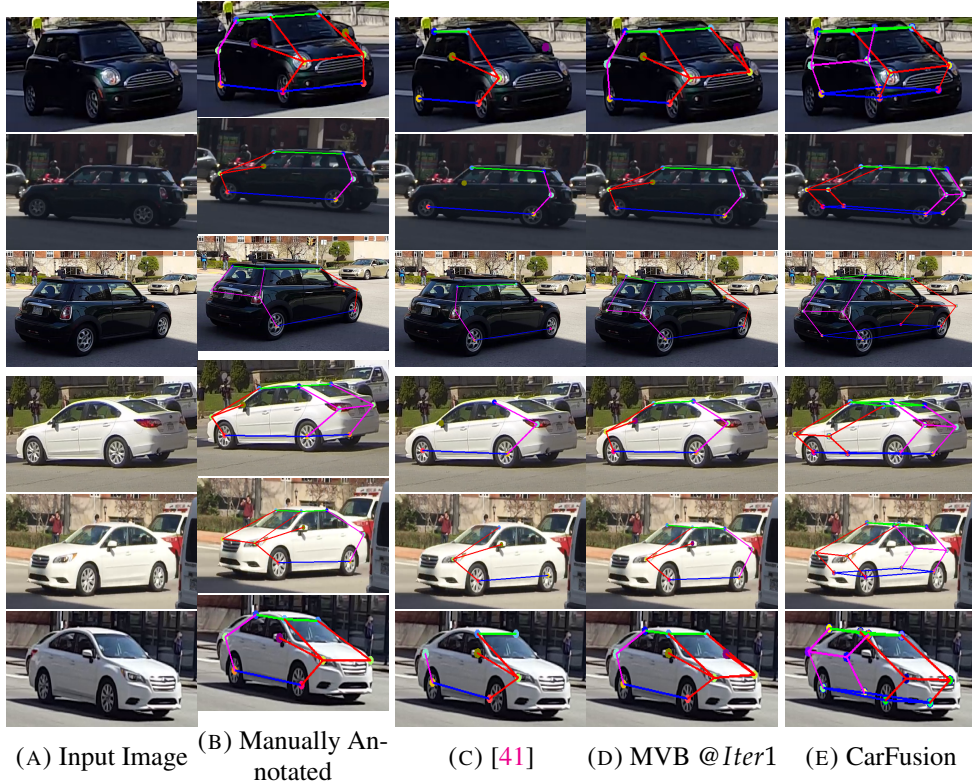
FIGURE 4.5: Qualitative analysis of the structured point detector before and after multiview bootstrapping (MVB), shown for two cars in three different views. Initial detectors were trained using Alejandro et al.[41]. The CarFusion approach was used to reconstruct the cars. Then the resulting 3D structured points were re-projected to all the views and used to retrain/bootstrap the detectors. The MVB approach shows clear visual improvement over the baseline, even in the presence of occlusions.
