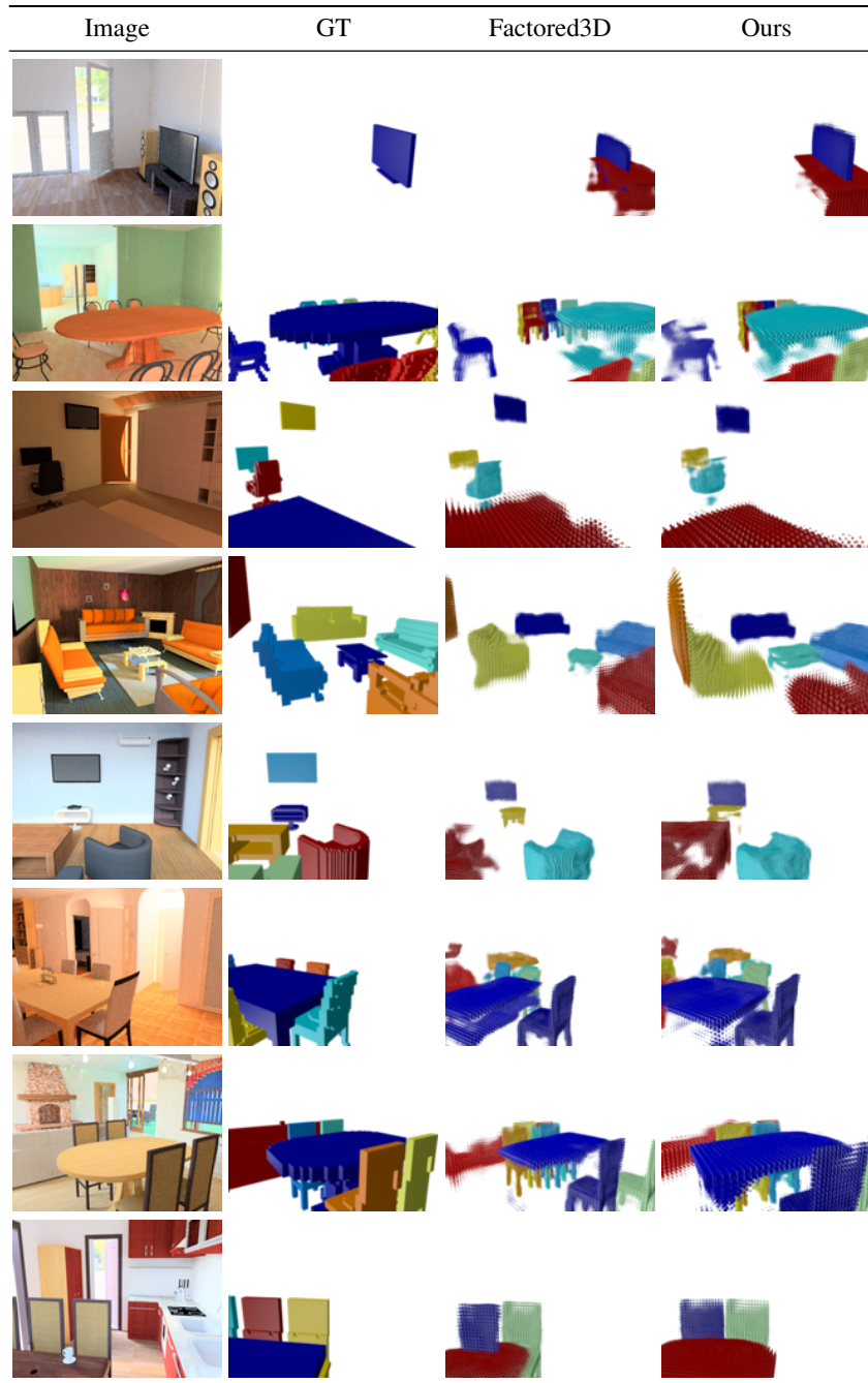
Figure 3.5: Detection Setting for SUNCG: We visualize sample prediction results in the detection setting (Section ??). Our method produces better estimates than the baseline, e.g. , in the first image the television set and the table are better placed. The colors only indicate separate instances, and do not correspond between the ground-truth and the predicted representations. We show 3D outputs (detection setting) for NYU in the supplementary material
