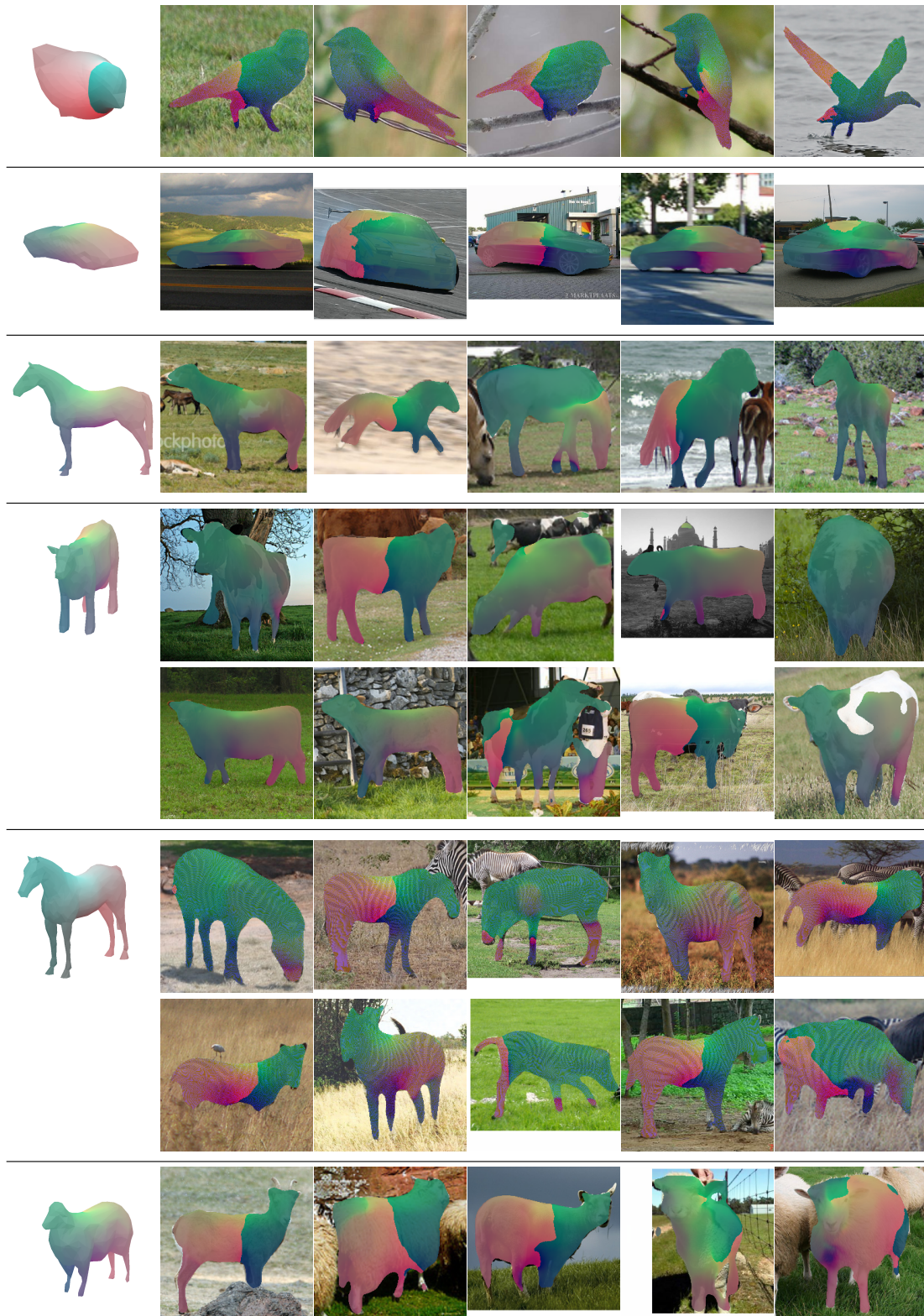
Figure 2.6: Predicted Canonical Surface mapping for six different categories. The color at each image pixel depicts the color at the corresponding surface point on the 3D template shape in the left row. While the predictions are mostly accurate, some error modes include: a) inferring globally incorrect CSM due to pose ambiguity (e.g. third horse), or b) incorrect local predictions due to missing segmentation (e.g. last cow).
