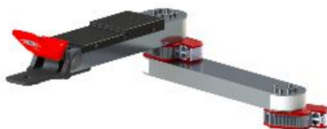
Figure 4.1: Rendering of two DOF arm mounted on vertical slide of ground robot.
