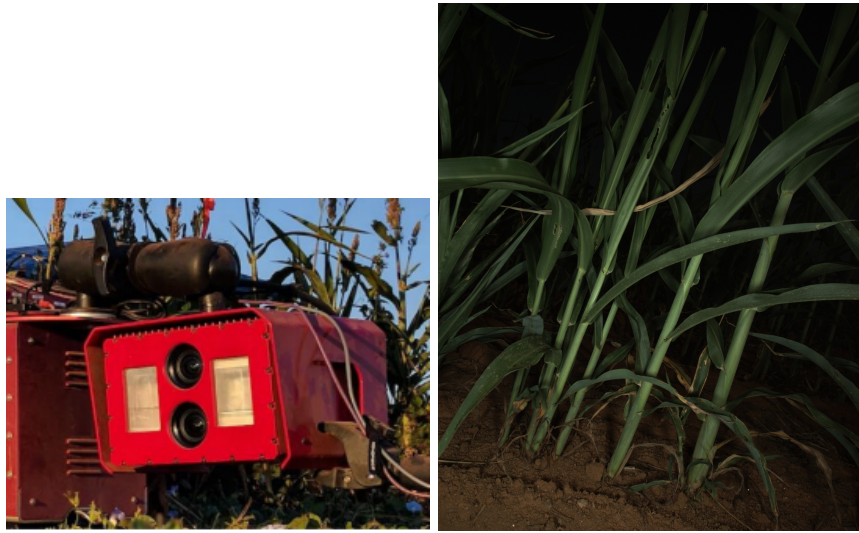
Figure 3.2: Left: The robot navigating in a Hop field. Left: The custom built stereo imager. Right: Sample image of sorghum with active lighting.
