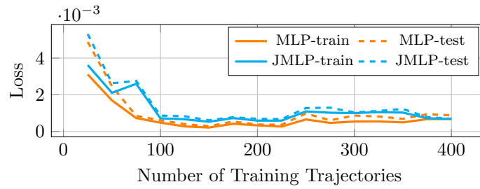
Figure 9.4: Loss versus number of training trajectories for the cartpole MLP. Although the both models perform about equally well on instantaneously predicting the discrete dynamics, the sample efficiency and performance on the closed-loop control problem different significantly (see Figure 9.2b.)
