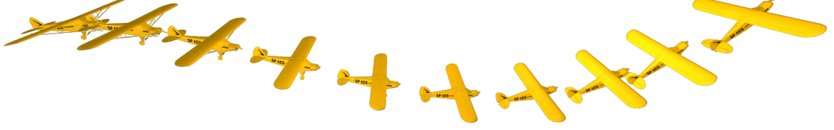
(a) Expert perching demonstration, a high angle-of-attack maneuver that minimizes velocity at the goal position with complex, post-stall aerodynamic forces
