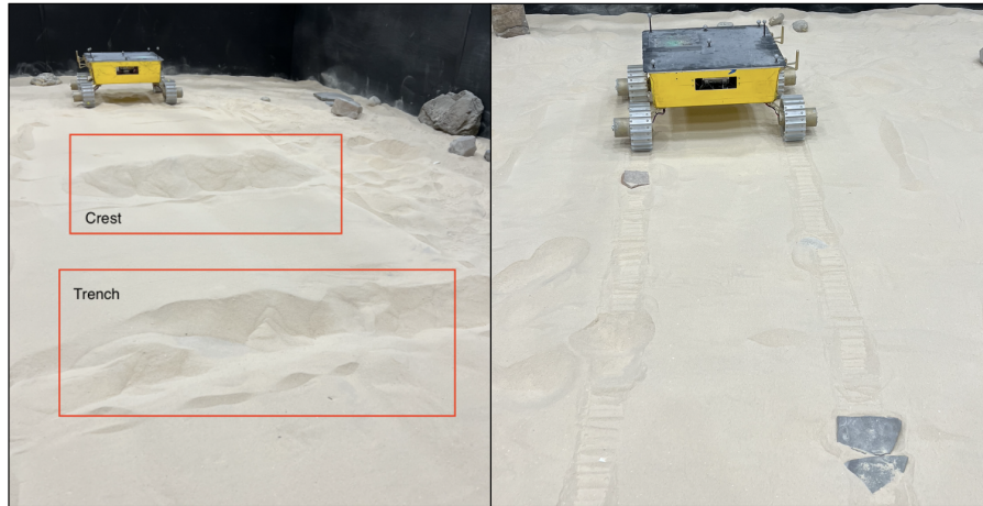
Figure 5.9: Morphin going over a crest and trench (left) and embedded rocks (right)
