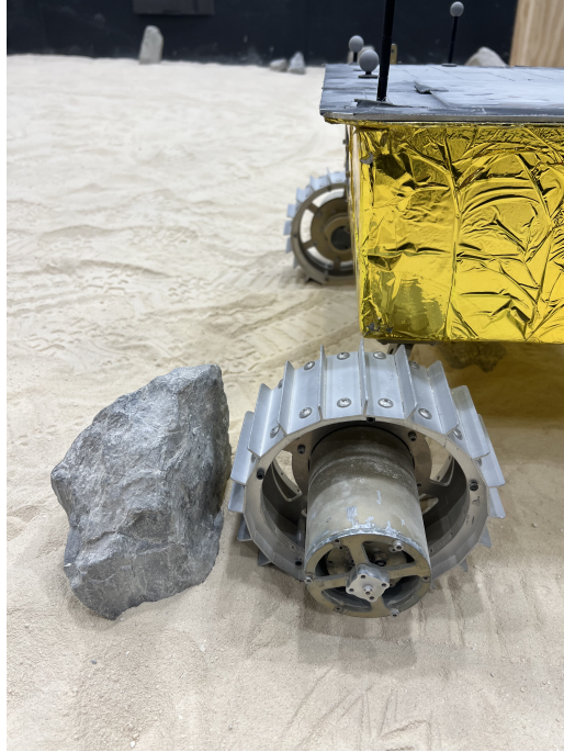
Figure 7.1: Morphin’s wheel up against a rock that is too steep to surmount
