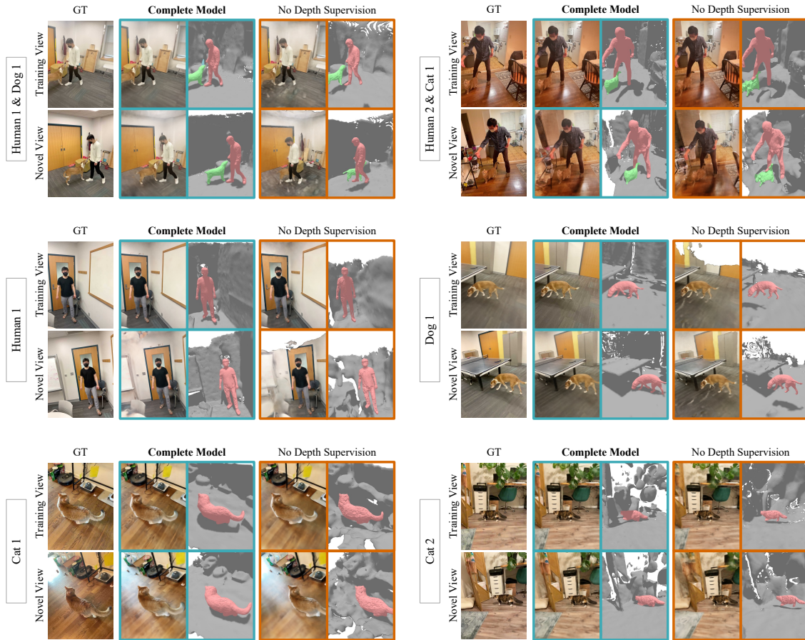
Figure F.1: Ablation Study on Depth Supervision. While removing depth supervision from Total-Recon (COMPLETE MODEL) doesn't significantly hamper the training-view RGB renderings, it induces the following failure modes in the novel-view 3D reconstructions. (a) Floating objects : for the HUMAN 1 & DOG 1, DOG 1, HUMAN 1, and CAT 2 sequences, the foreground objects float above the ground, as evidenced by their shadows. (b) Objects that sink into the background : for the HUMAN 2 & CAT 1 sequence, the reconstructed cat is halfway sunk into the ground. (c) Incorrect occlusions : for the HUMAN 1 & DOG 1 sequence, the human is incorrectly occluding the dog. (d) Lower reconstruction quality : for the HUMAN 2 & CAT 1 sequence, the cat displays lower reconstruction quality, and, for all sequences except HUMAN 1 & DOG 1 and CAT 2, the background object exhibits lower reconstruction quality. [Videos]
