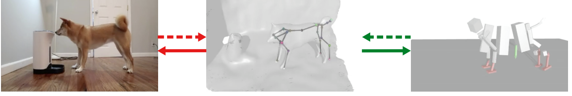
Figure 2.3: The physics-informed 3D reconstruction pipeline: Differentiable rendering from a monocular video (left) and differentiable physics simulation (right) update key-point motion estimates (middle). Solid red and green arrows represent rendering and physics-roll-out costs; dashed arrows are corresponding gradients.
