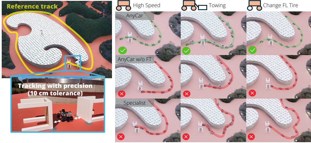
Figure 4.1: Performance of AnyCar and baselines in the wild under state estimation errors. Above: A 10 cm tolerance corridor is set as a checkpoint. Below: each row represents the true trajectory of one method, and each column corresponds to a specific setting for the 1/16 scale car: high speed (2 m/s), towing a box, and replacing the front left tire with a plastic wheel. All settings significantly alter the vehicle dynamics.
