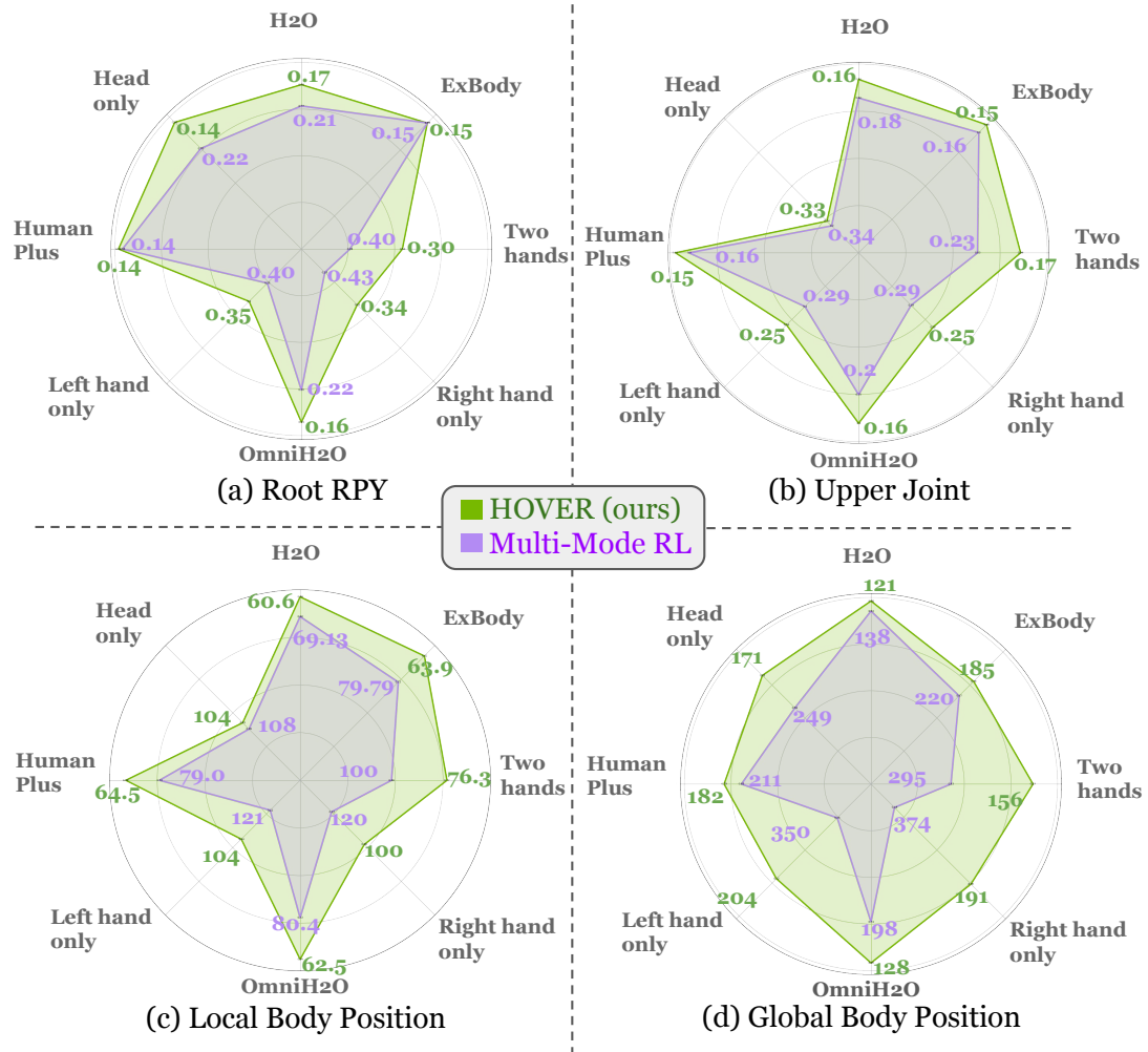
Figure 2.4: We assess the tracking accuracy of two multi-mode control policies— HOVER (ours) (green) and Multi-Mode RL (purple)—across eight distinct humanoid control modes. The comparison is visualized across four key performance metrics in the radar charts.
