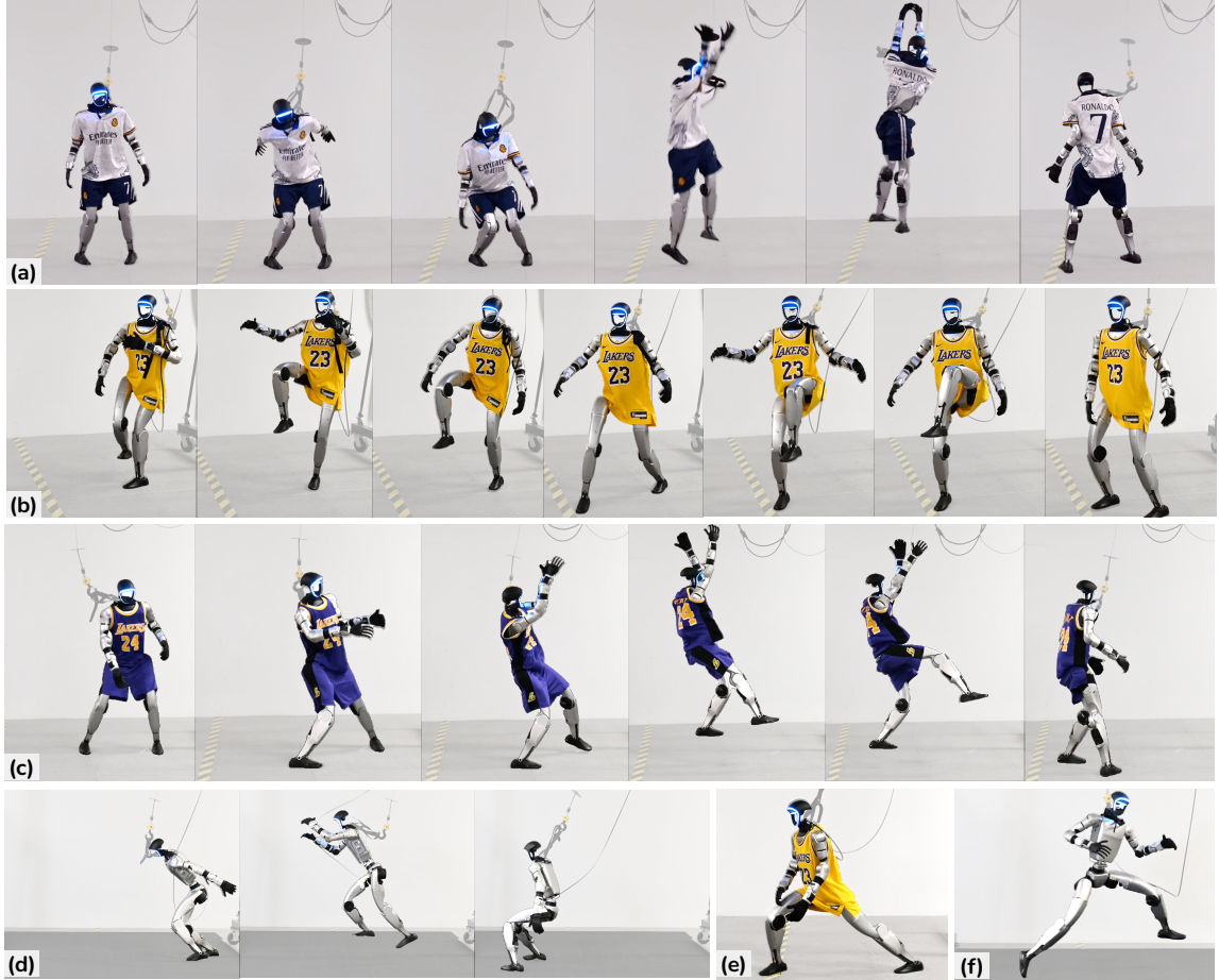
Figure 1.2: The humanoid robot (Unitree G1) demonstrates diverse agile whole-body skills, showcasing the control policies' agility: (a) Cristiano Ronaldo's signature celebration involving a jump with a 180-degree mid-air rotation; (b) LeBron James's "Silencer" celebration involving single-leg balancing; and (c) Kobe Bryant's famous fadeaway jump shot involving single-leg jumping and landing; (d) 1.5m-forward jumping; (e) Leg stretching; (f) 1.3m-side jumping.
