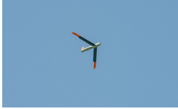
Figure 4.20: Fixed-wing platform used for autonomous flights with an onboard camera pitched at 10 degrees [189]
