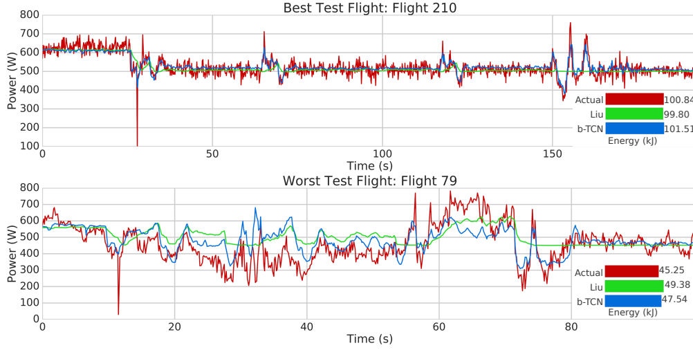
Figure 7.4: Test Flights with the best and worst MAPE for b-TCN. The bar graphs in the bottom right corners represent the total energy estimate over the entire flight.
