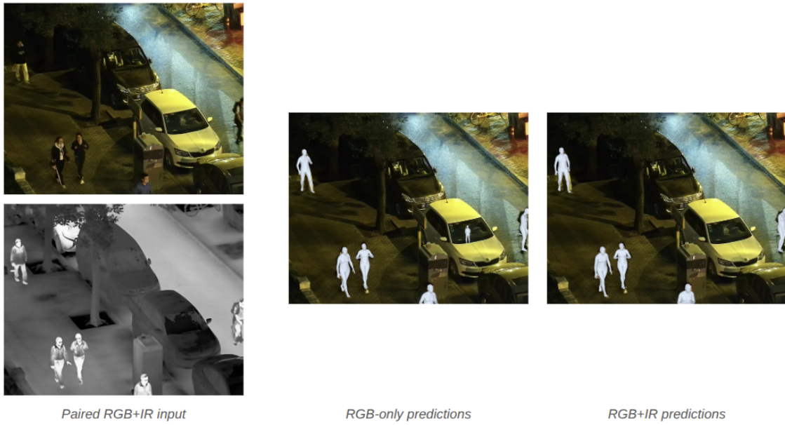
Figure 5.2: RGB+IR fusion improves pose recovery for occluded and poorly lit pedestrians.
