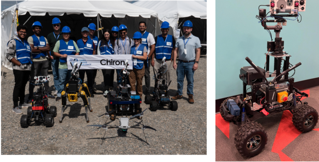
Figure 1.2: (Left) Team Chiron at DTC Challenge Year-1 with our (pet) robots. (Right) A closer look at the sensor payload used in Year-1. We used an iPhone as our primary RGB sensor attached to a gimbal for necessary movements. We also utilized Zed cameras for locomotion, speaker/microphone for specific tasks, with the main computational overhead being handled by an onboard Nvidia Jetson Orin.
