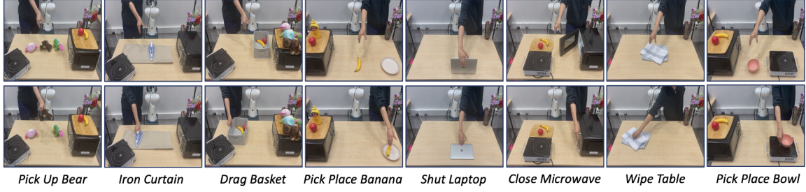
Figure 4.4: Real-world manipulation tasks. Human demonstrations for the eight evaluation tasks, shown as two frames per task. Tasks span prehensile and non-prehensile manipulation, including grasping, pushing, closing, wiping, and placing.
