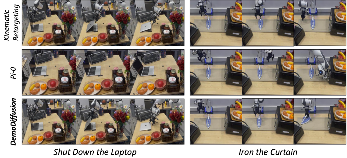
Figure 4.6: Qualitative comparisons for real-robot manipulation. Rollout progressions (start, intermediate, final frame) for two tasks. Kinematic retargeting (top) produces plausible motion but loses contact before completing the task. Pi-0 (middle) performs general reaching but fails to manipulate the correct object. DemoDiffusion (bottom) reaches the object and maintains contact through task completion. See the project page for full videos.
