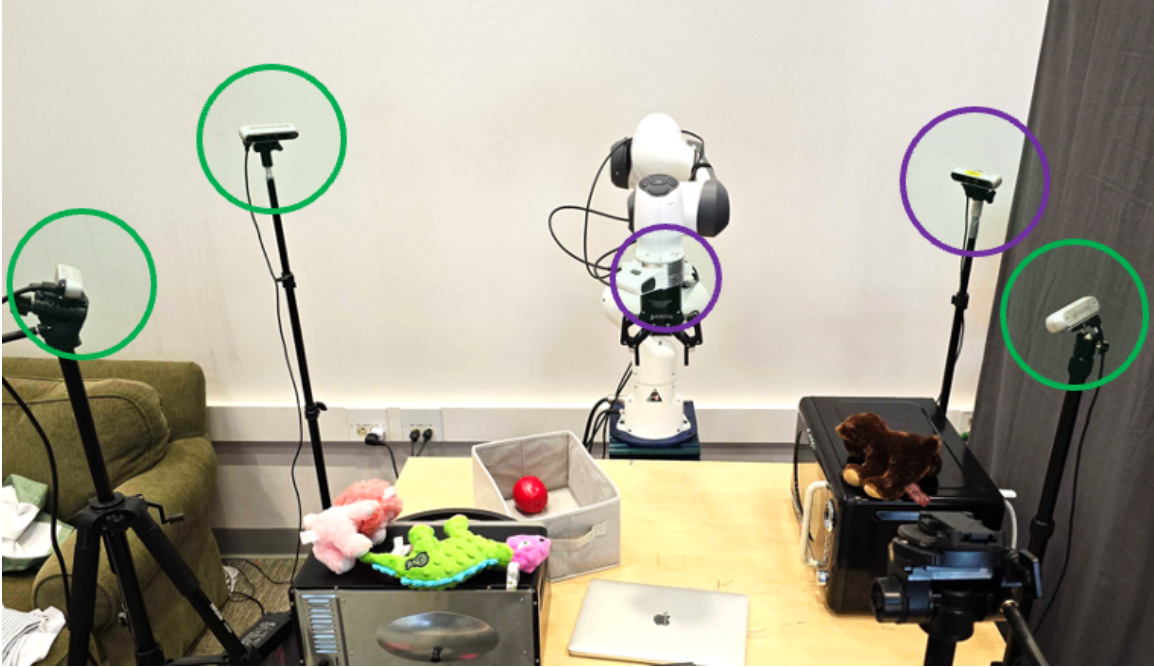
Figure 4.5: Workspace with five cameras. We use the four external cameras for triangulation to obtain the global pose of the hand mesh from a human demonstration. The pre-trained policy uses the two cameras marked in purple.
