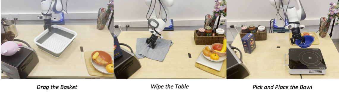
Figure A.2: Zero-shot generalization to new objects. We evaluate DemoDiffusion ’s generalization capabilities to new objects on 3 tasks – drag the basket, wipe the table, and pick and place the bowl. While the objects have different colors and shapes from those of the objects in the human demonstration, DemoDiffusion adjusts its behavior to these new objects. Please refer to the website for detailed visualizations.
