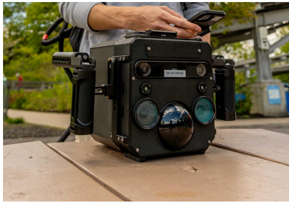
Figure 3.1: TartanStar Payload. Consists of Stereo RGB, Stereo Thermal, Radar, LIDAR, IMU, GPS, and Stereo Event
