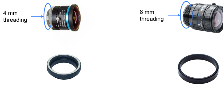
Figure 3.2: Lens thread length comparison. The standard 4 mm threaded C-mount lens uses the included 5 mm ring adapter, while the 8 mm threaded Basler lens requires an additional 5 mm spacer before mounting onto the EVK4’s CS-mount body.
