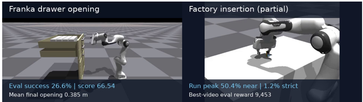
Figure 3.8: Representative learned policies. Drawer opening exhibits coherent reach-and-pull behavior, whereas plug insertion approaches the target but remains limited by fine-grained alignment and contact.
