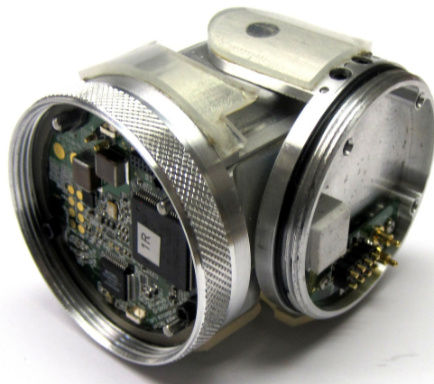
Fig. 1: Photo of a prototype SEA Snake Module. The module is 5 cm (2 in.) in diameter and provides a 1-DOF rotary motion of \pm 90^\circ . The module contains a rubber-based series elastic actuator that can output over 6 N-m of torque.
