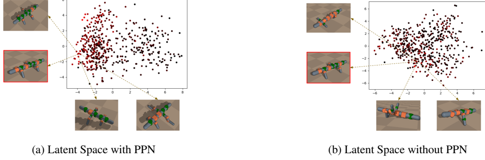
Figure 3: Visualization of two different latent spaces (a) when the VAE is co-trained with the property predictor, and (b) without the property predictor. Here we project the latent points into a two-dimensional space, for visualization purposes, by taking the first two principal components. The color of the points correspond to its performance for a given task (here, traversing flat terrain), where a darker color denotes worse performance. We additionally show designs neighboring the same robot (with red border) in the two different latent spaces. We can see that the addition of the property predictor implicitly encourages designs with similar performance to be grouped together, which we find results in more efficient optimization.
