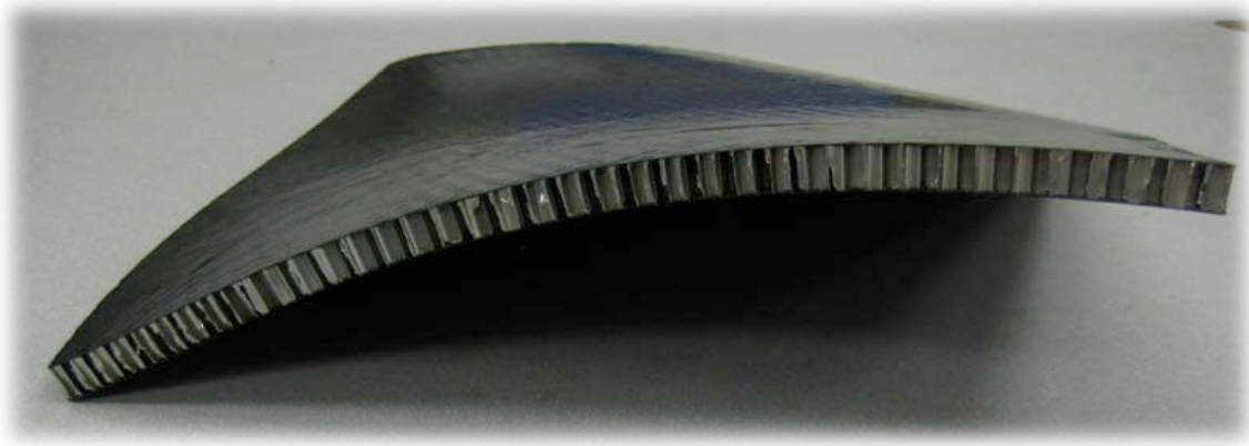
Figure 39: Carbon-honeycomb chassis design makes use of carbon face sheets to handle tensile loads and aluminum honeycomb to resist bending.
