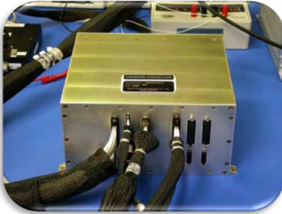
Figure 45: Low mass COTS avionics chassis
