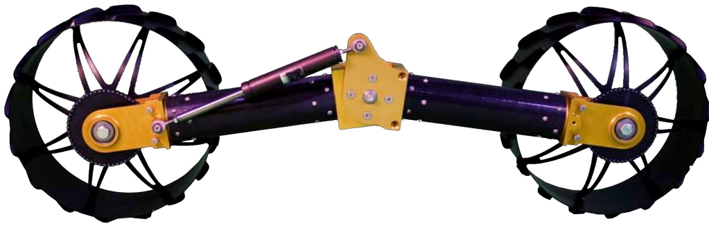
Figure 29: Mobility sidearm drives two wheels with a single actuator at the shoulder and roller chain to transmit torque to wheels.
