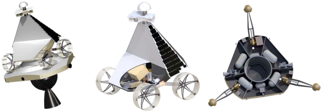
Figure 11: Devised conjoined lander-rover configuration; avionic components reside in the rover; the lander is only a pallet with propulsion appended.
