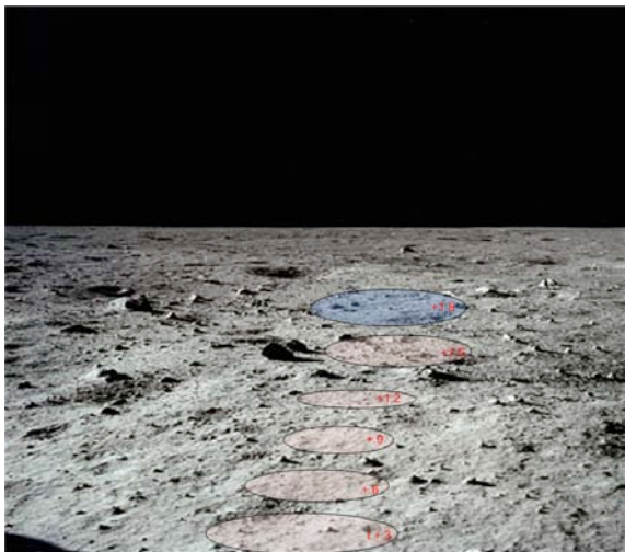
Figure 18: Rover trajectory is overlaid on camera views based on predictive modeling.
