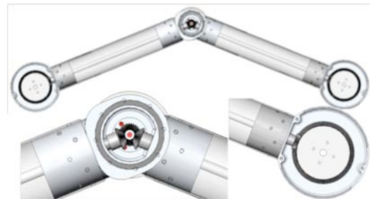
Figure 28: Miter gear sidearm configuration transmits torque to wheels through a complex gearing system.
