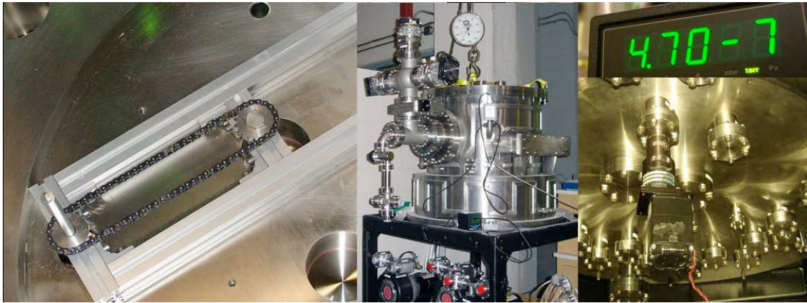
Figure 29: Testing roller chain in vacuum.
