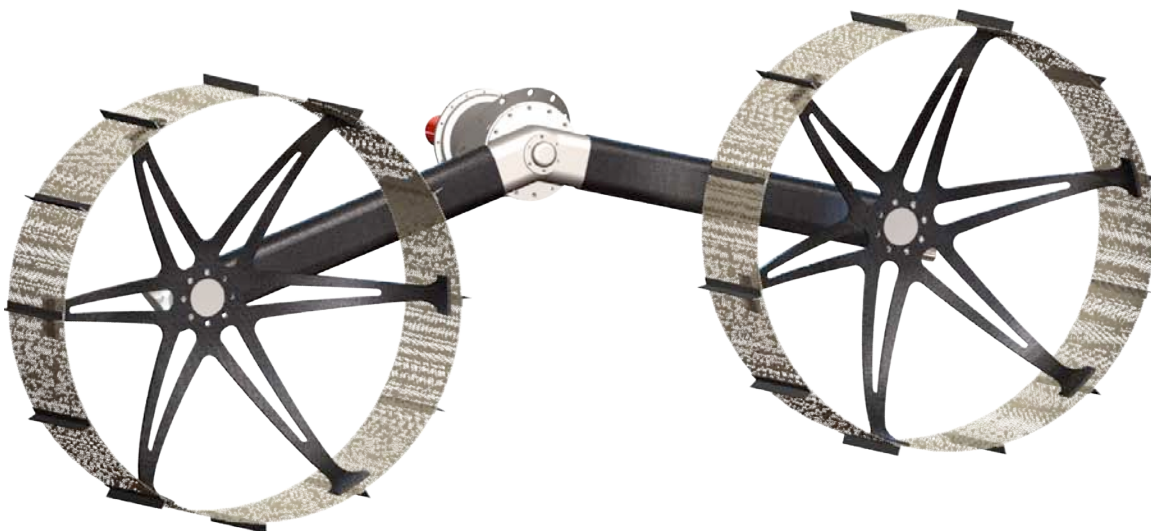
Figure 30: Mobility mass reduced through analysis of load conditions.
