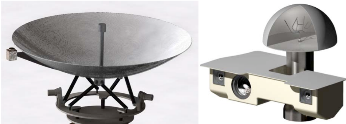
Figure 23: One design uses a steerable antenna guided by a small camera. The XPrize rover succeeds with a low mass stationary evolved antenna.
