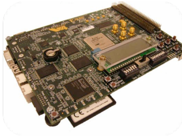
Figure 47: Custom motor control board utilizes FPGAs to minimize componentry.
