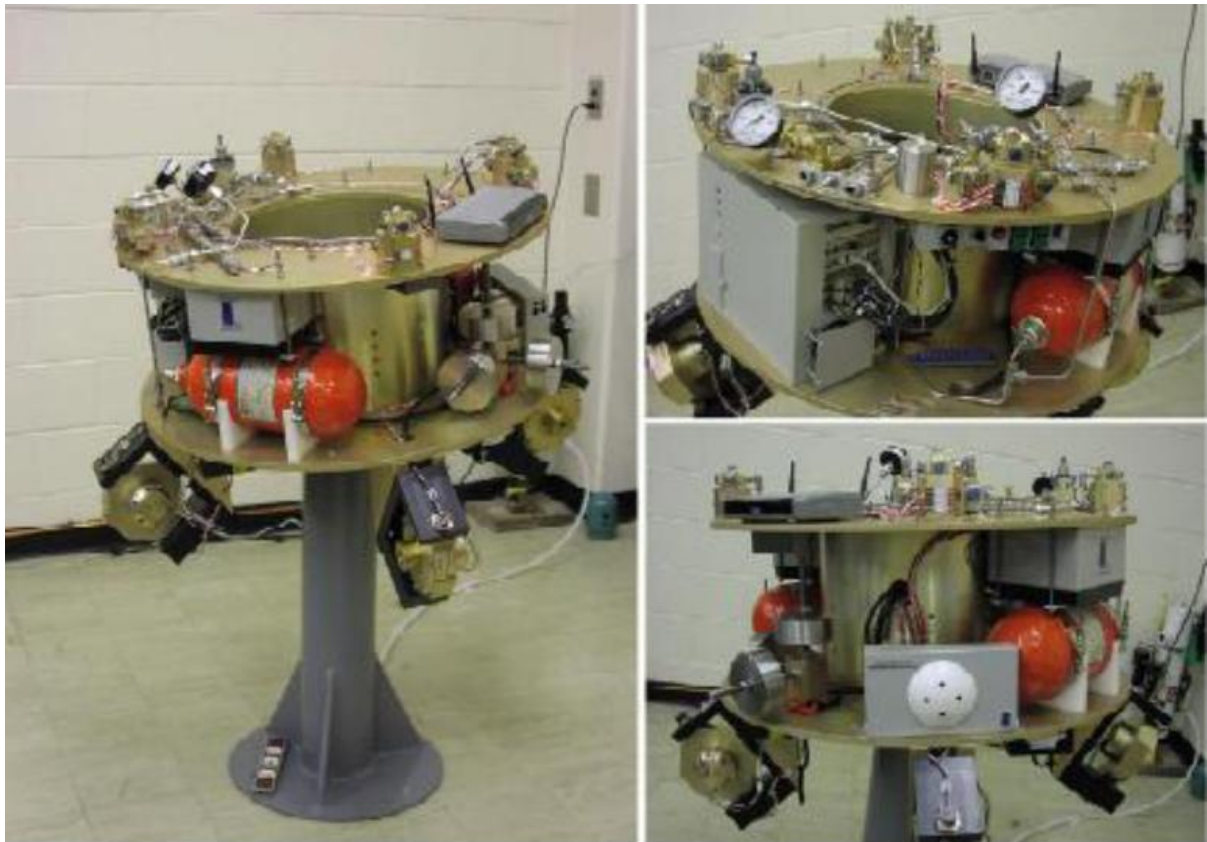
Figure 7: GIT's experimental test-bed for integrated attitude dynamics and control research
