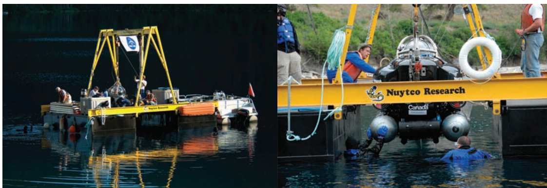
Figure A1. DeepWorker launch platform (barge), showing submersible deployment under way (left) (photo by: Jim Thompson); and DeepWorker deploying through barge moon pool (right) (photo by: Matthew Deans).
