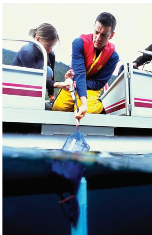
Figure 6. Margarita Marinova and Bernard Laval conducting CTD (conductivity temperature depth) and Licor (light sensor) casts in Pavilion Lake. (Photo by: Donnie Reid.)
