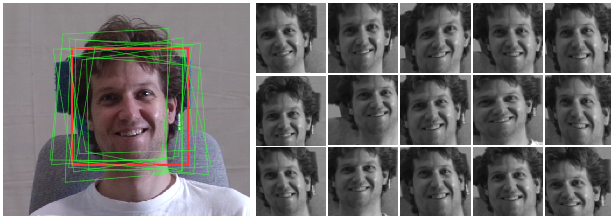
Figure 5.1: Visualization of the perturbed samples \mathcal{S} = \{\Delta \mathbf{p}_n, \mathcal{I}_n(\mathbf{p}_n \circ \Delta \mathbf{p}_n)\}_{n=1}^N used for training the SDM, Conditional LK, and Generative LK methods. Left: the original source image, where the red box is the ground truth and the green boxes are perturbed for training. Right: examples of the synthesized training samples.
