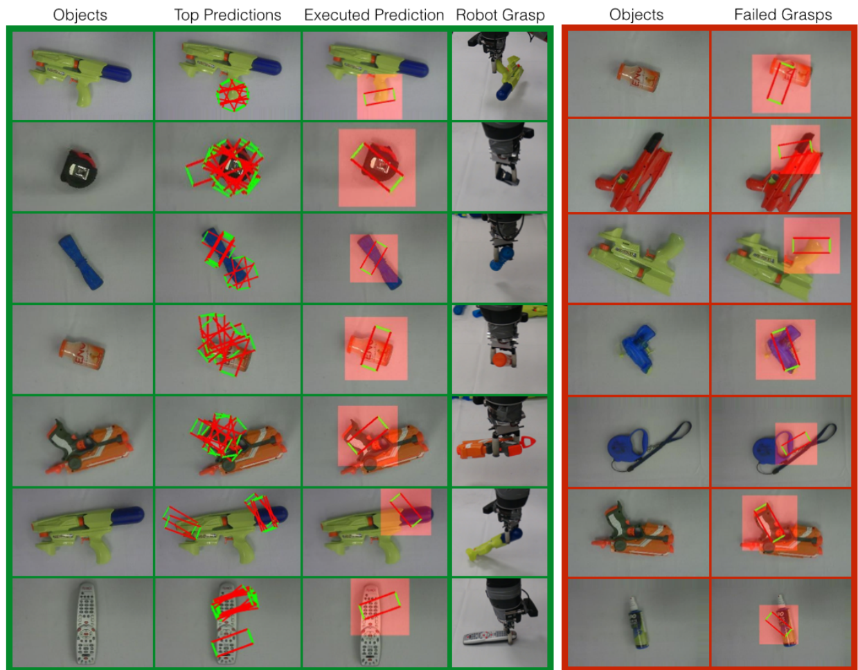
Fig. 10. Grasping Test Results: We demonstrate the grasping performance on both novel and seen objects. On the left (green border), we show the successful grasp executed by the Baxter robot. On the right (red border), we show some of the failure grasps. Overall, our robot shows 66% grasp rate on novel objects and 73% on seen objects.
