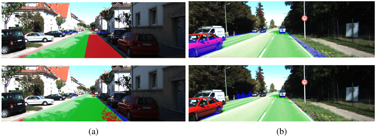
Figure 2.6: Successful cases for the automatic labeling of images. Top row displays results after initial map projection and bottom row shows results after our label refinement approach. In (a), our approach is able to extend the road annotation to cover the whole road. In (b), we successfully removed the incorrectly labeled cars from the road class. The color coding is as follows: Green - True Positive, Red - False Negative, Blue - False Positive for road.
