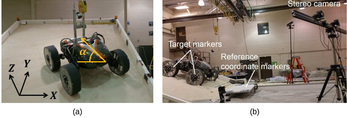
Figure 3.3: Setup of the slope-ascent experiments. (a) The rover was placed on the slope at an angle of attack \alpha by using a crane. (b) The stereo camera captures the target markers on the wheels and a software compute their positions with respect to the reference coordinate markers.
