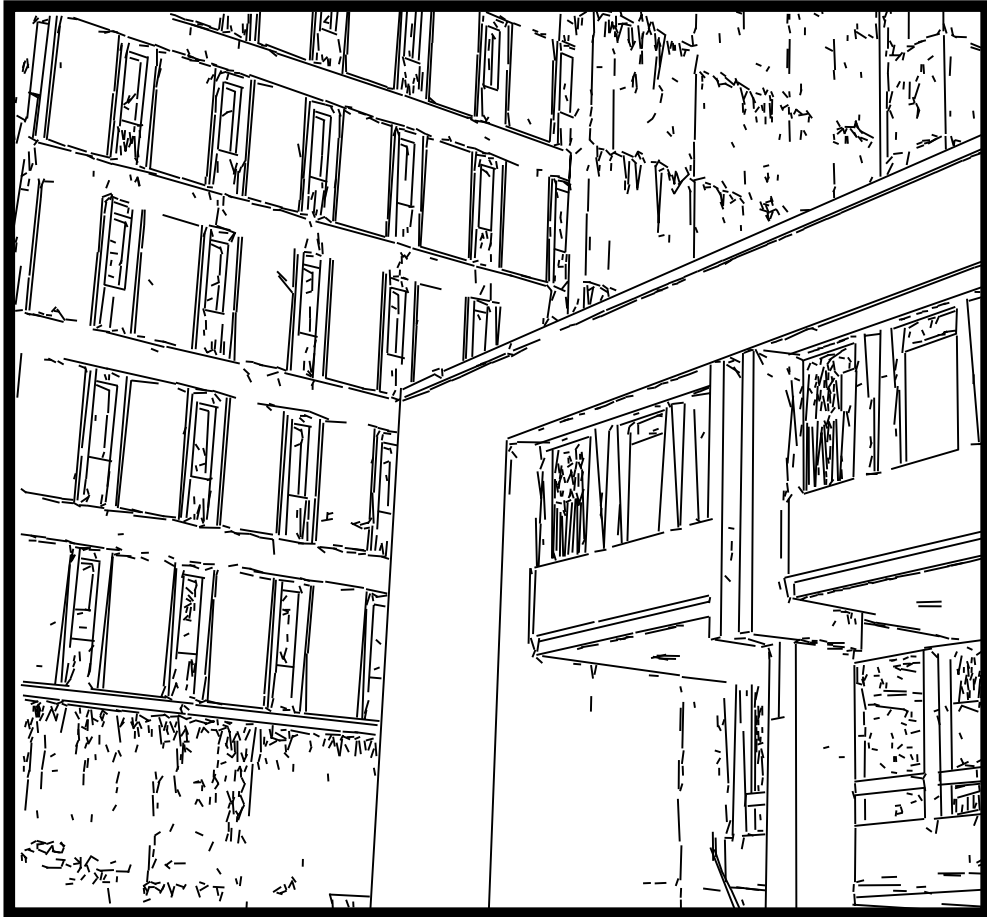
Figure 4.1: Straight line segments from an outdoor building scene. These line segments were computed by the Boldt straight line extraction algorithm [Boldt89]. There were 2372 lines extracted for this image.
