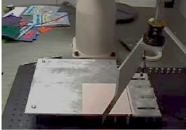
Figure 4.9: A machine that can fold simple origami.
