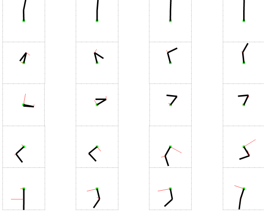
Fig. 5. Best trajectory for 2-link pendulum at every 0.1 sec.
